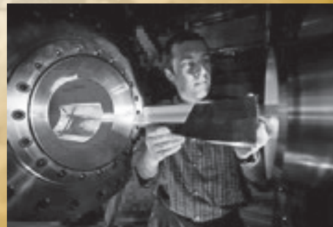
Tom Juliano installs a Hyper-2000 model onto the sting of the Mach 6 wind tunnel operated at Purdue University
