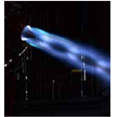
This gaseous oxygen/kerosene high pressure rotating detonation combustor is currently under study at the Maurice J. Zucrow Laboratories.
