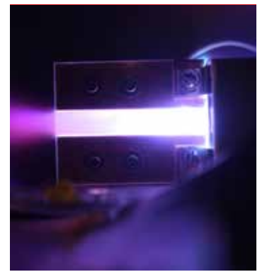
A liquid-fed pulsed plasma accelerator is currently studied at the Applied Plasma Science Laboratory.
