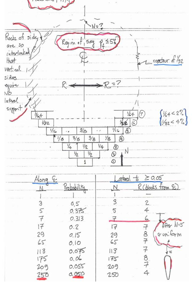
volume on "Earth Tunneling with Steel Support." The test results led to the following conclusions regarding the prerequisites for arch action and the factors which determine the load on the roof support in tunnels through crushed rock and cohesionless sand located above the water table.
