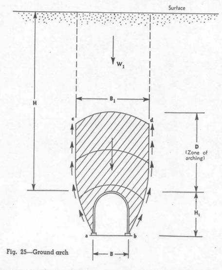
tends to move into the tunnel. This movement is resisted by the friction along the lateral boundaries a c and b d of this mass. The friction forces transfer the major part of the weight of the overburden, with height H onto the material located on both sides of the tunnel and the roof support carries only the balance, equivalent to a height  $H_{\rm p}$ .
