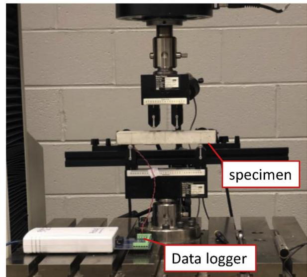
Fig. 2. The setup for 4-pt bending test.
