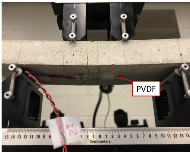
Fig. 1. 4-point flexural test specimen.
