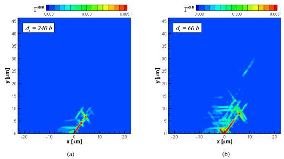
**Figure 11**: Contours of total slip  $\Gamma = \sum |\gamma^{(\alpha)}|$  (contributed only by the dislocations) around the crack tip at  $K_l/K_0 = 0.08$  for two cases with different slip plane spacing: (a)  $d_s = 240 \text{ b}$ , (b)  $d_s = 60 \text{ b}$ . Note the difference in the plastic zone  $(r_p)$  between the two cases.
