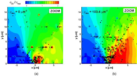
(a) (b) **Figure 5**: <u>Zoom (15 x 15 µm)</u> showing the normalized stress and dislocation distribution at  $K_1/K_0 = 0.08$  for the two limiting cases: (a)  $\rho_{obs} = 0 \mu m^{-2}$ , (b) $\rho_{obs} = 103.4 \mu m^{-2}$
