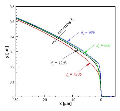
**Figure 13**: Crack shape at  $K_l/K_0 = 0.08$  for different slip plane spacing.
