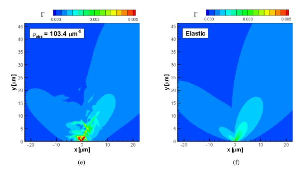
**Figure 6 (cont.)**: Contours of total slip  $\Gamma = \sum |\gamma^{(\alpha)}|$  around the crack tip at  $K_I/K_0 = 0.08$ . (a)  $\rho_{obs} = 0$   $\mu m^{-2}$ , (b)  $\rho_{obs} = 8.4 \ \mu m^{-2}$  (c)  $\rho_{obs} = 25.4 \ \mu m^{-2}$  (d)  $\rho_{obs} = 51.7 \ \mu m^{-2}$  (e)  $\rho_{obs} = 103.4 \ \mu m^{-2}$  (f) Elastic solution.
