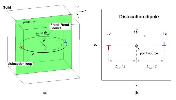
**Figure 2**: In two dimensions the dislocation loop is projected into the plane and modeled by a dislocation dipole. The Frank-Read source is modeled by a point source given by the projection of the real source into the plane *x-y*.
