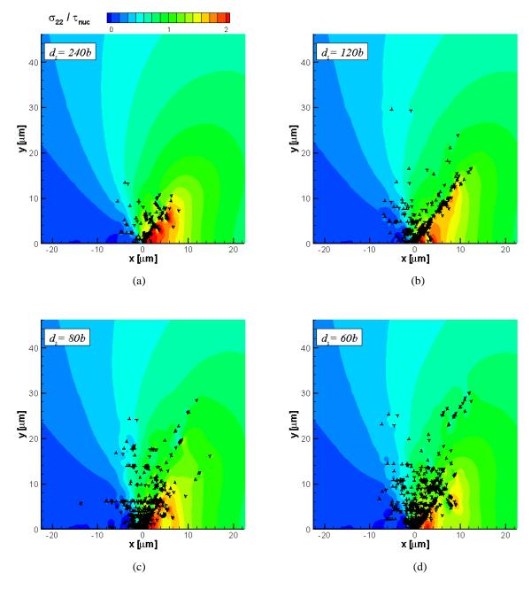
**Figure 9:** Normalized opening stress  $\sigma_{22}/\sigma_{max}$  and dislocation distribution at  $K_l/K_0 = 0.08$  for different slip planes spacing: (a)  $d_s = 240 \text{ b}$ , (b)  $d_s = 120 \text{ b}$ , (c)  $d_s = 80 \text{ b}$ , and (d)  $d_s = 60 \text{ b}$ .
