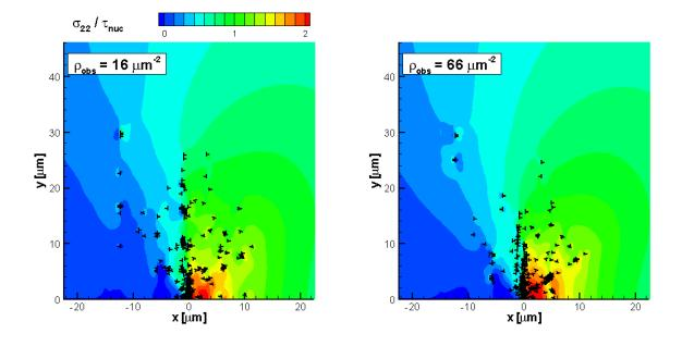
**Figure 14:** Normalized opening stress  $\sigma_{22}/\sigma_{max}$  and dislocation distribution at  $K_1/K_0 = 0.08$  for the bcc-like orientation and two different obstacle densities: (a)  $\rho_{obs} = 16 \ \mu m^{-2}$ , (b)  $\rho_{obs} = 66 \ \mu m^{-2}$ .
