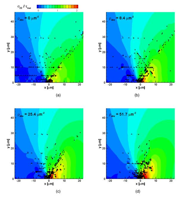
**Figure 4**: Normalized opening stress  $\sigma_{22}/\tau_{nuc}$  and dislocation distribution at  $K_I/K_0 = 0.08$ . (a)  $\rho_{obs} = 0$   $\mu m^{-2}$ , (b)  $\rho_{obs} = 8.4 \ \mu m^{-2}$  (c)  $\rho_{obs} = 25.4 \ \mu m^{-2}$  (d)  $\rho_{obs} = 51.7 \ \mu m^{-2}$  (e)  $\rho_{obs} = 103.4 \ \mu m^{-2}$  (f) Elastic solution.
