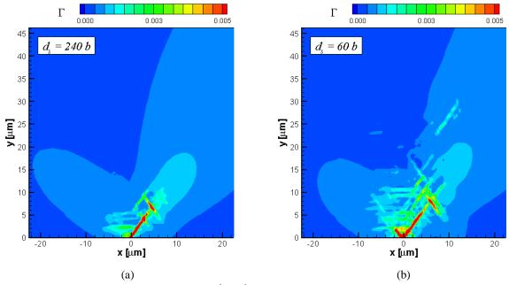
**Figure 10:** Contours of total slip  $\Gamma = \sum |\gamma^{(\alpha)}|$  around the crack tip at  $K_l/K_0 = 0.08$  for two cases with different slip plane spacing: (a)  $d_s = 240$  b, (b)  $d_s = 60$  b.
