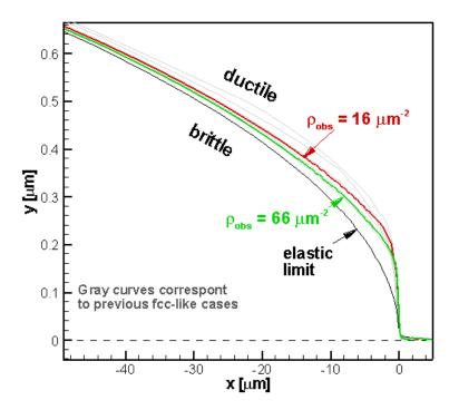
**Figure 17**: Crack shape at  $K_l/K_0 = 0.08$  for the bcc-like orientation and two different obstacle densities.
