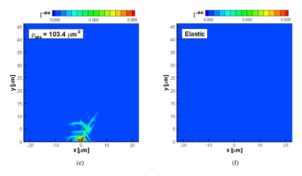
**Figure 7(cont.)**: Contours of total slip  $\Gamma = \sum |\gamma^{(\alpha)}|$  (contributed only by the dislocations) around the crack tip at  $K_1/K_0 = 0.08$ . (a)  $\rho_{obs} = 0 \ \mu m^{-2}$ , (b)  $\rho_{obs} = 8.4 \ \mu m^{-2}$  (c)  $\rho_{obs} = 25.4 \ \mu m^{-2}$  (d)  $\rho_{obs} = 51.7 \ \mu m^{-2}$  (e)  $\rho_{obs} = 103.4 \ \mu m^{-2}$  (f) Elastic solution.
