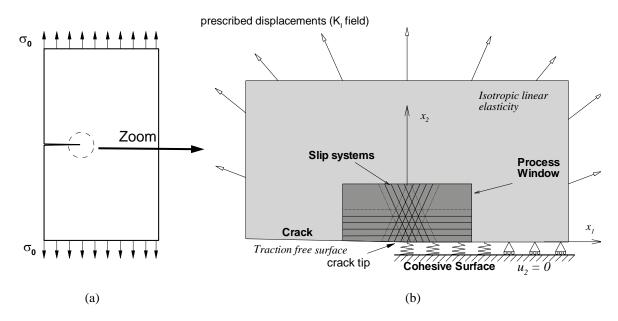
**Figure 1**: Mode I crack analysis with the discrete dislocation model and cohesive interfaces. Because of symmetry, only half the problem needs to be analyzed.
