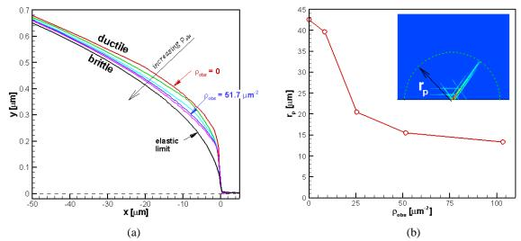
**Figure 8**: (a) Variation of Crack shape at  $K_l/K_0 = 0.08$  with Obstacle Density. (b) Plastic zone size  $(r_p)$  vs obstacle density at  $K_l/K_0 = 0.08$ .
