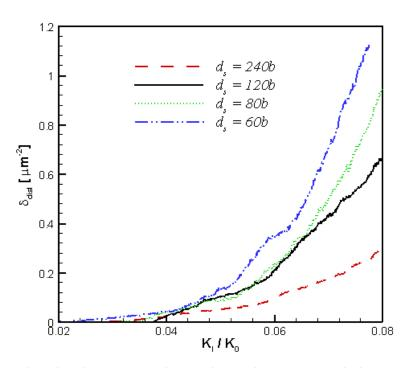
**Figure 12**: Dislocation density measured over the entire process windows versus the normalized applied stress intensity factor  $K_I/K_0$  for the different slip plane spacing for an FCC-like material.
