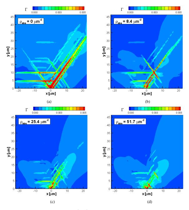
**Figure 6**: Contours of total slip  $\Gamma = \sum |\gamma^{(\alpha)}|$  around the crack tip at  $K_l/K_0 = 0.08$ . (a)  $\rho_{obs} = 0 \ \mu m^{-2}$ , (b)  $\rho_{obs} = 8.4 \ \mu m^{-2}$  (c)  $\rho_{obs} = 25.4 \ \mu m^{-2}$  (d)  $\rho_{obs} = 51.7 \ \mu m^{-2}$  (e)  $\rho_{obs} = 103.4 \ \mu m^{-2}$  (f) Elastic solution.
