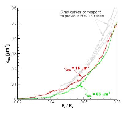
**Figure 18:** Dislocation density measured over the entire process windows versus the normalized applied stress intensity factor  $K_I/K_0$  for the fcc-like (gray) and bcc-like orientations (red and green) with two different obstacle densities.
