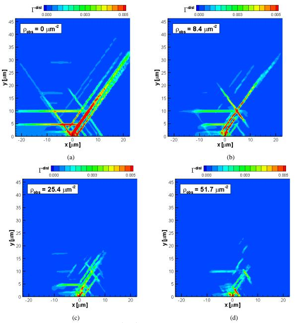
(c) (d) **Figure 7**: Contours of total slip  $\Gamma = \sum |\gamma^{(\alpha)}|$  (contributed only by the dislocations) around the crack tip at  $K_I/K_0 = 0.08$ . (a)  $\rho_{obs} = 0 \ \mu m^{-2}$ , (b)  $\rho_{obs} = 8.4 \ \mu m^{-2}$  (c)  $\rho_{obs} = 25.4 \ \mu m^{-2}$  (d)  $\rho_{obs} = 51.7 \ \mu m^{-2}$  (e)  $\rho_{obs} = 103.4 \ \mu m^{-2}$  (f) Elastic solution.
