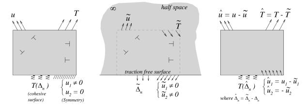
**Figure 3**: Decomposition of the problem into the problem of interacting dislocation in the homogeneous free-traction half space (~ fields) and the complementary problem of the elastic body without dislocations (^ fields).
