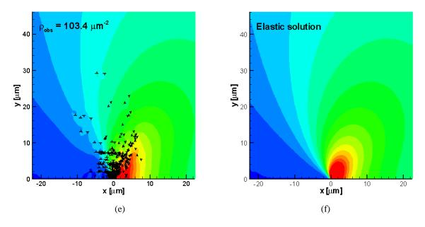
**Figure 4 (cont.)**: Normalized opening stress  $\sigma_{22}/\tau_{nuc}$  and dislocation distribution at  $K_l/K_0 = 0.08$ . (a)  $\rho_{obs} = 0 \ \mu m^{-2}$ , (b)  $\rho_{obs} = 8.4 \ \mu m^{-2}$  (c)  $\rho_{obs} = 25.4 \ \mu m^{-2}$  (d)  $\rho_{obs} = 51.7 \ \mu m^{-2}$  (e)  $\rho_{obs} = 103.4 \ \mu m^{-2}$  (f) Elastic solution.
