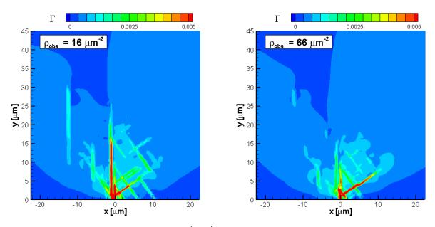
**Figure 15**: Contours of total slip  $\Gamma = \sum |\gamma^{(\alpha)}|$  around the crack tip at  $K_l/K_0 = 0.08$  for the bcc-like orientation and two different obstacle densities: (a)  $\rho_{obs} = 16 \ \mu m^{-2}$ , (b)  $\rho_{obs} = 66 \ \mu m^{-2}$ .
