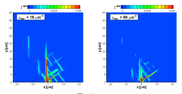
**Figure 16**: Contours of total slip  $\Gamma = \sum |\gamma^{(\alpha)}|$  (contributed only by the dislocations) around the crack tip at  $K_l/K_0 = 0.08$  for the bcc-like orientation and two different obstacle densities: (a)  $\rho_{obs} = 16 \mu m^{-2}$ , (b)  $\rho_{obs} = 66 \mu m^{-2}$ .
